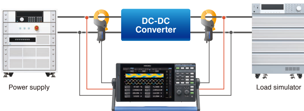
Efficiency testing in development and production
