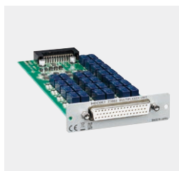
MULTIPLEXER UNIT Z3003
