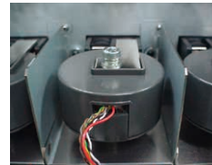
DCCT current sensor (in the PW3337)
