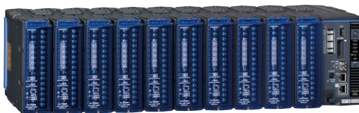
LR8102 main unit with ten M7100 Voltage/ Temp modules (sold separately) attached
