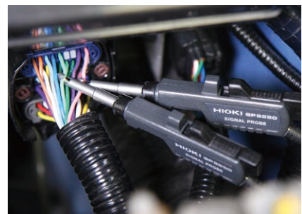
Undamaged wires for easy and safe measurement
