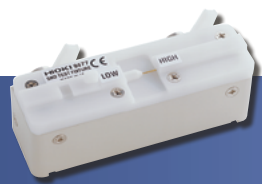
SMD TEST FIXTURE 9677 Electrodes on the side; DC to 120MHz, measurable sample sizes: 0402 to 0603 (EIA), 1005 to 1608 (JIS)
