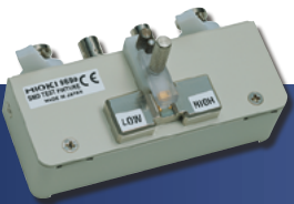
SMD TEST FIXTURE 9699 Electrodes on the bottom; DC to 120MHz, measurable sample sizes: 0608 to 0805 (EIA), 1608 to 2012 (JIS)
