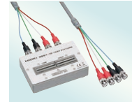
TEST FIXTURE 9261-10 Cable length 1 m (3.28 ft), DC to 8 MHz, impedance characteristics of 50 Ω, 4-terminal pair configuration, measurable conductor diameter: \phi 0.3 (0.01 in.) to 1.5 mm (0.06 in.)
