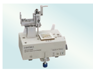
SMD TEST FIXTURE IM9100 Direct connection type, SMDs with electrodes on the bottom, DC to 8 MHz, metric (inch): 0402(01005), 0603(0201), 1005(0402)
