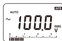
Measuring 100 V using the 300 V range
