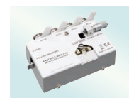
SMD TEST FIXTURE IM9110 Direct connection two-terminal measurement type for measuring SMDs, DC to 1 MHz, measurable sample sizes: 008004 (inch)
