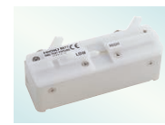
SMD TEST FIXTURE 9677 Direct connection type, For measuring SMDs with electrodes on the side; DC to 120 MHz, test sample dimensions: 3.5 mm \pm 0.5 mm (0.14 in. \pm 0.02 in.)
