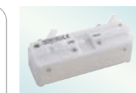
SMD TEST FIXTURE 9677 Direct connection type, For measuring SMDs with electrodes on the side; DC to 120 MHz, test sample dimensions: 3.5 mm \pm 0.5 mm (0.14 in. \pm 0.02 in.)
