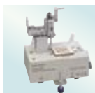
SMD TEST FIXTURE IM9100 Direct connection type, SMDs with electrodes on the bottom, DC to 8 MHz, metric(inch): 0402(01005), 0603(0201), 1005(0402)
