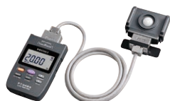
Sensor unit and main display can be separated. Sold separately
