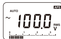
Measuring 100 V using the 300 V range
