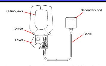
The clamp sensor and secondary coil are marked to indicate the direction of current flow, to ensure that the measurement current and output current have the same phase.
