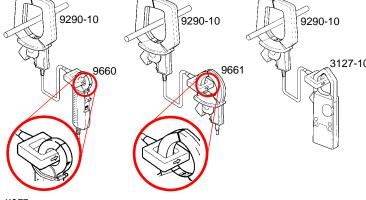
The effect of conductor positioning of the clamp sensor clamped to the secondary coil should be considered. Please verify the specifications of the clamp sensor being used.
