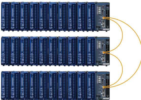
Example of synchronized measurement with 3 loggers
