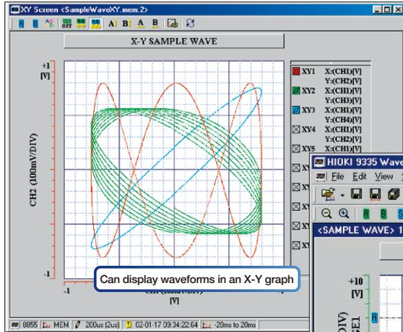
The Wave Processor 9335 lets you load binary files from a MEMORY HiCORDER and then check the waveform or measured results on the waveform display screen and the numeric display screen. The 9335 also supports the memory recorder X-Y display function. The waveform display screen and the X-Y display screen also can be split into graphs for each channel.
