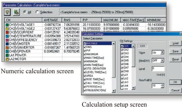
19 types of numerical calculations can be displayed for all the areas or a specific area only. In addition to effective value, maximum value, frequency, and other standard values, you can also calculate values for characteristics such as duty ratio and rise time.
